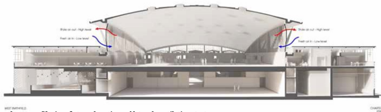
Dome clerestory Glazing- Internal section-- Natural ventilation strategy
